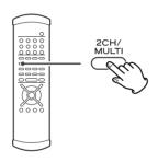
When playback is stopped, use the 2CH/MULTI button to select either 2CH (stereo) or MULTI (multi-channel surround) audio output from the analog outputs.
